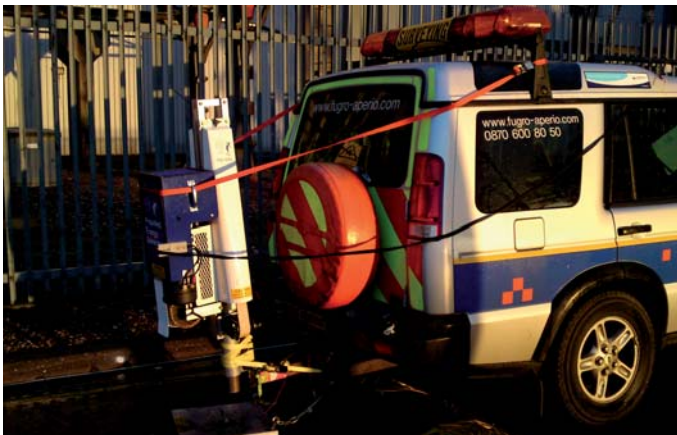
Figure 3: Higher power impulsive source (accelerated weight drop) on an industrial site.
