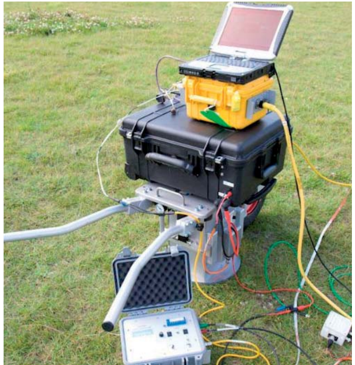
Figure 4: A high frequency vibroseis seismic source capable of transmitting compressional and shear wave energy used for investigations down to 50-100m.
