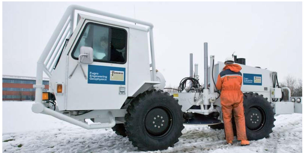
Figure 5: Swept-frequency seismic source (vibroseis) used for seismic surveys from tens of metres to beyond 1km in depth.
